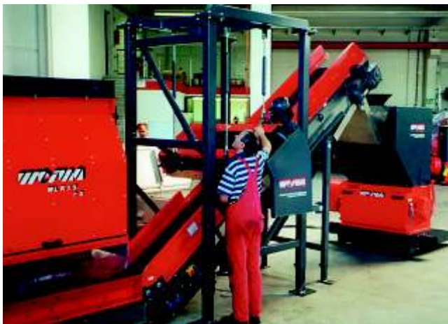
WLK/NZ – Side by Side version with magnetic separation
