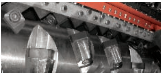
Can handle any material: the PreCut rotor.
