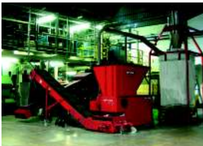
Closed Rotor Granulator of the NZ Series
