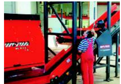
Open Rotor Granulator of the SMW Series
