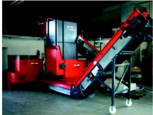
Horizontal Shredding System for long profiles and cut-offs prior to SMW
