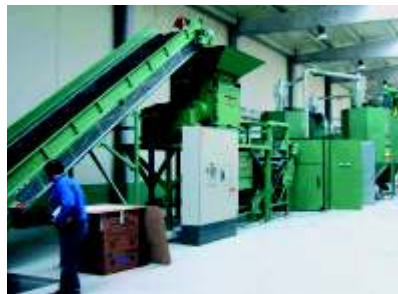
Open Rotor Granulator of the SMW Series
